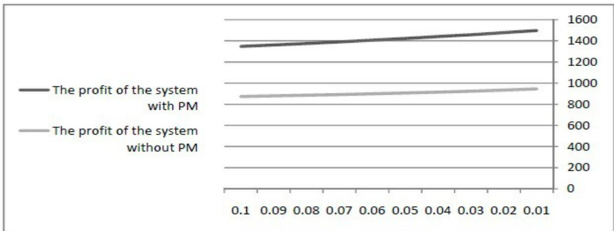
Fig. 4: Relation between the failure rate of type I and the expected total profit
