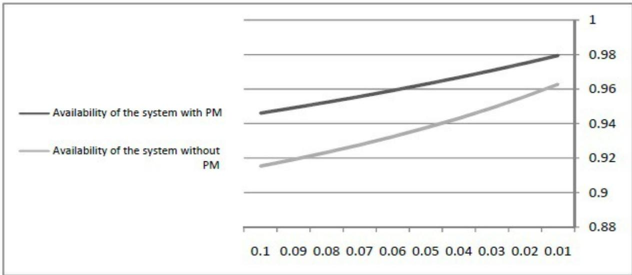
Fig. 3: Relation between the failure rate of type I and the Availability
